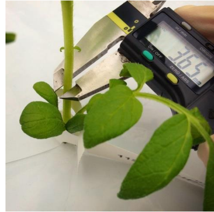
Measuring stem diameter with a digital caliper [shown here in aeroponics]
